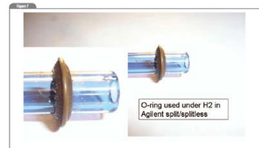
Figure 7: Deformation of "O"-ring when used with hydrogen as the carrier gas. Helium did not show this effect.
