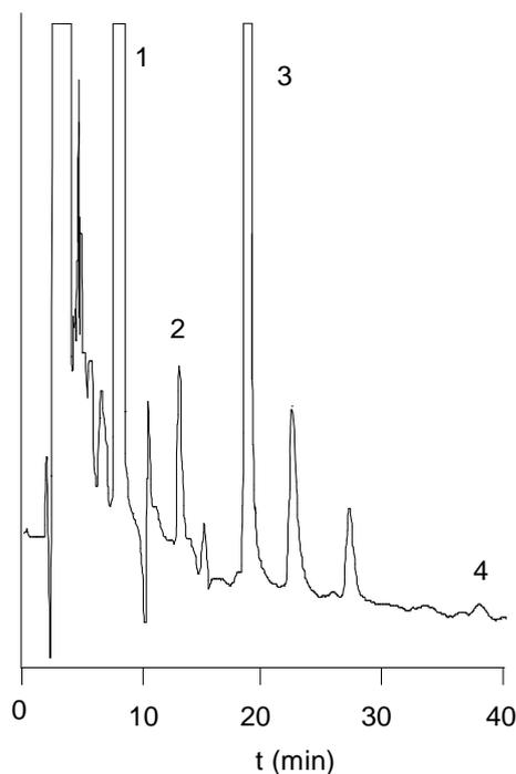
Fig. 1. Capillary LC of rat striatum dialysate. Concentrations and absolute amounts are: (1) Dopac 1  $\mu\text{mol/l}$  (64 fmole), (2) DA 5 nmol/l (5 amole), (3) HVA 0.23  $\mu\text{mol/l}$  (14 fmole) and (4) 5HT 3 nmol/l (0.18 fmole).
