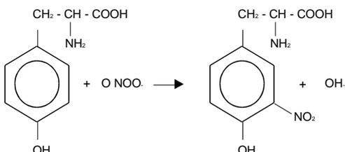
Fig. 1 Synthesis of 3-nitro-L-tyrosine from L-tyrosine and peroxynitrite.
