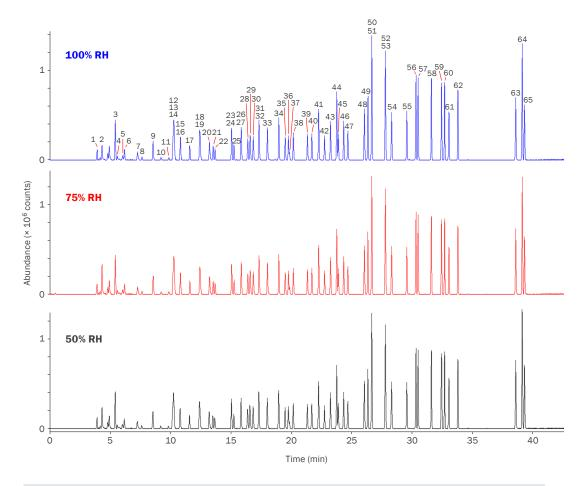
**Excellent peak shapes and interference-free monitoring** of early-eluting polar compounds (•) can be achieved using the UNITY-CIA *Advantage*-Kori-xr system, as shown by this analysis of a 65-component TO-15 mix at 50, 75 and 100% relative humidity.
