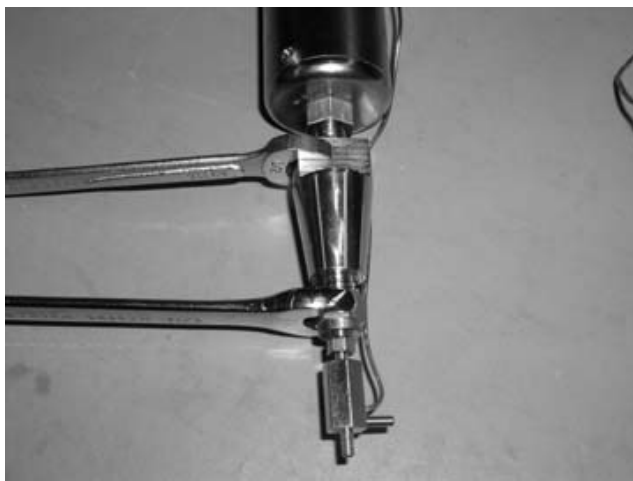
Figure 5 Tightening the Heater Swivel Nut
