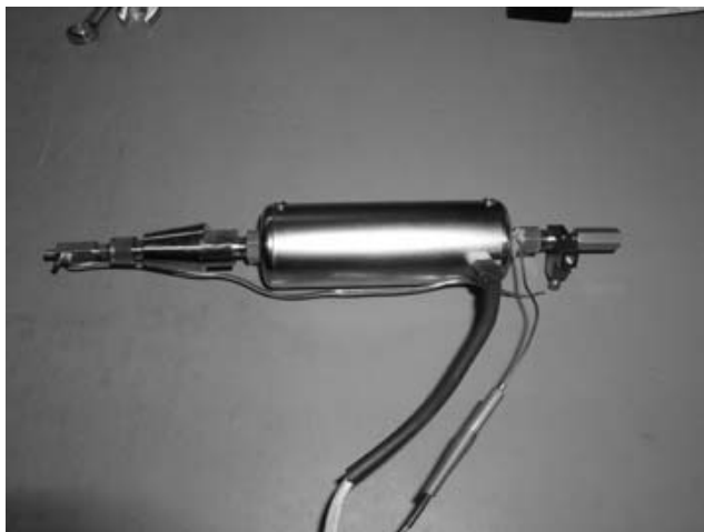
Figure 6 Proper Alignment of the Burner
