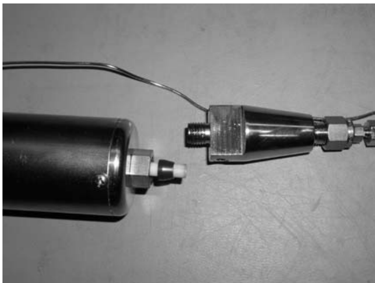
Figure 4 Large Ceramic Tube Properly Inserted into the Quartz Heater Assembly
