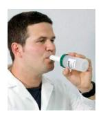
Markes International's Bio-VOC is a simple, disposable device for collecting alveolar (end-tidal) breath samples and transferring them quantitatively to sorbent tubes. It is used for non-invasive biological exposure monitoring of VOCs.
