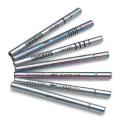
Clean tubes are essential for successful sampling. Make sure your tubes are contaminant-free by using Markes' TC-20 and TC-20 TAG tube conditioners – see page 14.
