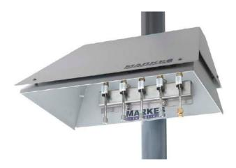
The 325 Field Station can accommodate up to five diffusive tubes for sampling of benzene and other hazardous VOCs, and is fully compatible with Markes' TubeTAG system (see page 15).
