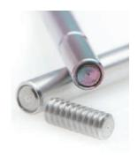
Markes' patented SafeLok tubes incorporate a diffusion-locking insert at each end, preventing sample loss or contamination.
