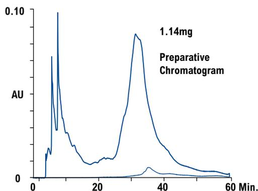
**Column:** Vydac® 219TP Diphenyl, 5µm, 4.6 x 250mm
