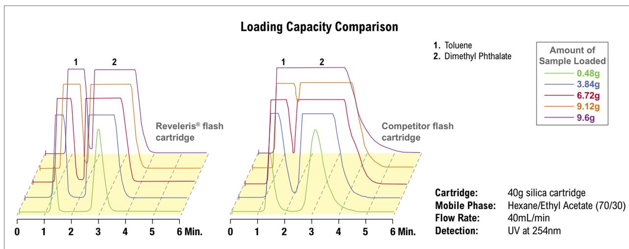
The Reveleris® flash cartridge maintains baseline resolution up to 9.12g, while a leading competitor cartridge only maintains resolution to 3.8g of load.
