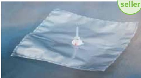
Combo valve gas sampling bags give the convenience and ease of a barbed on/off valve and a septum port combined into one fitting. The valve fitting features a 3/16" stem, which is suitable for use with most 1/4" tubing, and a sampling port. Bags are available in ALTEF and FEP.
