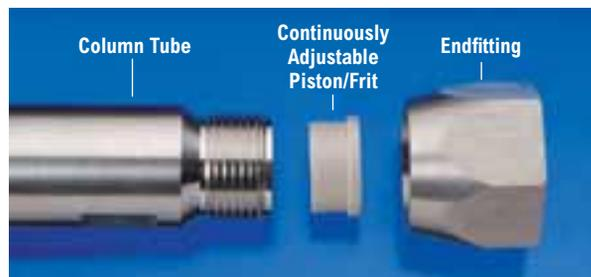
The easy-to-use preparative format has threaded endfittings and a continuously adjustable piston/frit. The piston/frit extends column life by compressing the packed bed to remove voids.
