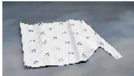
Cali-5-Bond™ gas sampling bags are constructed from inert 5.5mil thick material made from five layers of film. The layers are comprised of an inner layer of high-density polyethylene, followed by polyamide, an aluminum foil barrier, a polyvinylidene chloride layer and an outer layer of polyester.
