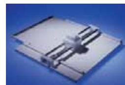
The TLC plate cutter has a high-quality carbide scriber mounted into a movable plastic head. It is designed to produce optimal scoring on the glass surface of 20 x 20cm TLC plates with a total thickness (glass + coating) of 2mm. A smaller template is included with the unit for ease in cutting 10 x 10cm plates.
