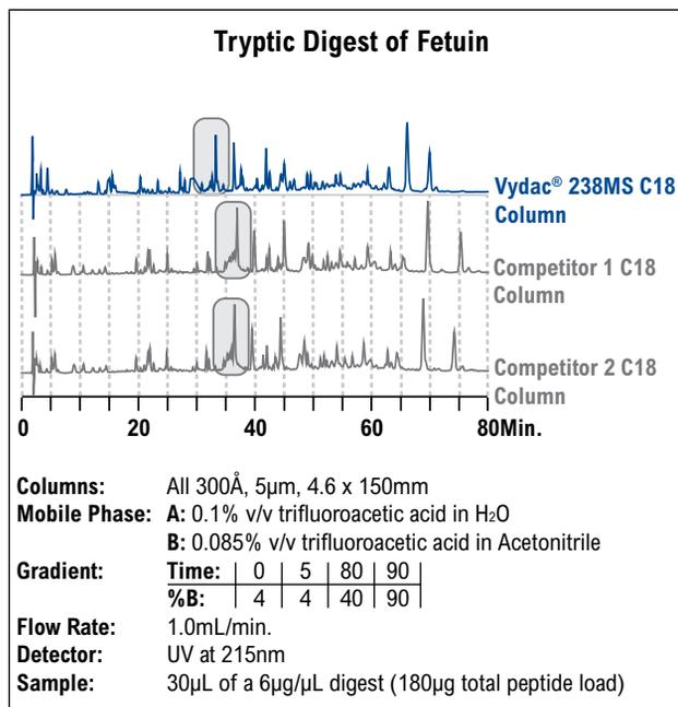
Sample components interfere with the separation of peptides on the Competitor 1 and 2 columns, appearing as a chromatographic “hump”. The unique selectivity of Vydac® MS columns solves separation problems.
