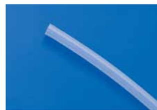
This low-pressure tubing has a double wall to prevent mobile phase regassing. The inert inner PTFE wall carries the mobile phase. The non-wetted outer wall is made from a translucent, flexible polymer with extremely low gas permeability. This low permeation tubing cuts regassing rates to negligible levels, while preserving PTFE's chemical resistance, visibility, and handling properties. Use with low permeation fittings kit.
