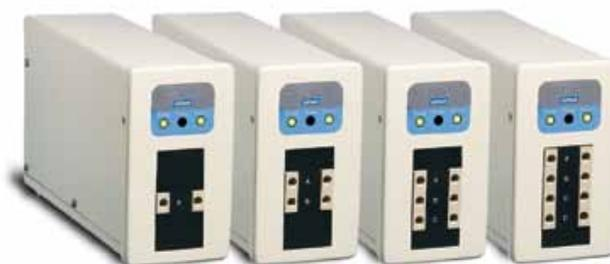
Flow rate instability and baseline noise are the likely result of dissolved air in the mobile phase. Eliminate these problems with the Alltech® on-line degassing system. Unlike helium sparging, degassing online does not require extra mobile phase preparation steps. Save time and avoid the expense, inconvenience and hazards associated with helium tanks.
