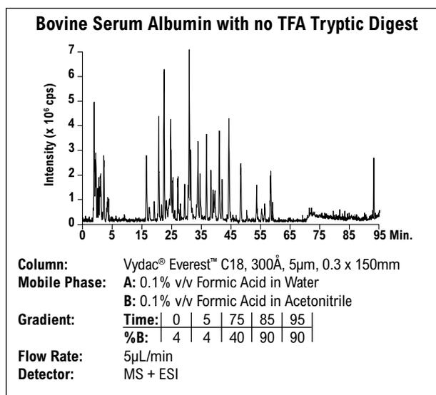
Everest™ columns outperform competitor columns by providing higher-resolution separations (average of 17% higher peak counts than competitor columns tested).
