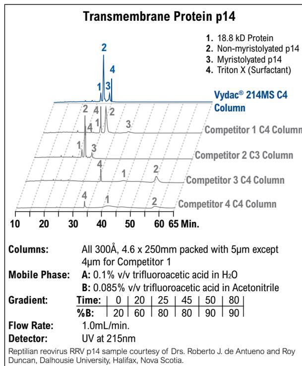
The Vydac® column provides better performance for this highly hydrophobic membrane protein (RRV p14) and its fatty acid modified (myristoylated) form.
