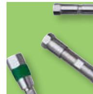
Prevail™ HPLC columns offer exceptional versatility for difficult separations. Traditional reversed-phase packings experience bonded phase collapse under highly aqueous (>95%) conditions. Prevail™ bonded phases remain fully extended in 100% aqueous and offer a high carbon load for exceptional retention at 100% organic. Retain both polar and non-polar compounds simply by adjusting the mobile phase.
