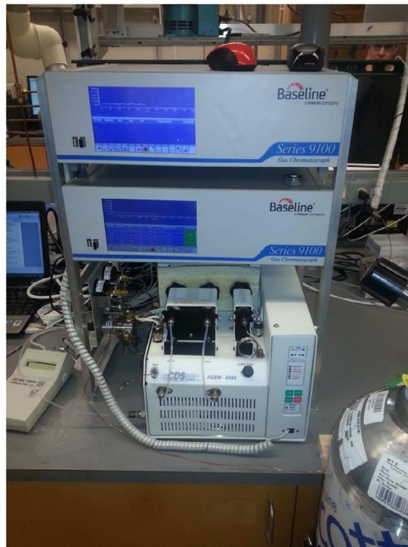
Figure 3: CDS ACEM 9350 with Baseline 9100 dual detector system
