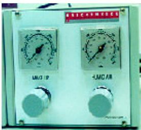
Make-up feeding (Nitrogen) with pressure control switch from 0 to 300kPa
