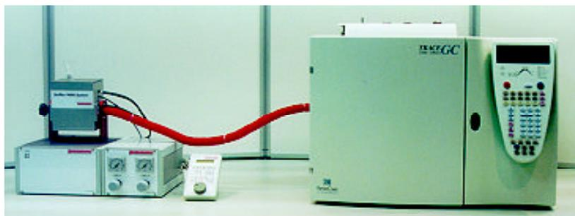
The Sniffer 9000 System is designed to be a dedicated „Sniffing-Device“ as a stand alone unit to be connected to any GC available on the market.
