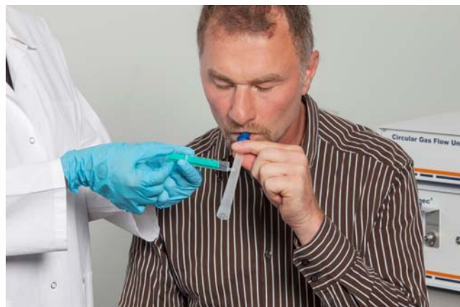
Figure 1: Manual sampling option: Exhaled breath is sampled into a reservoir (syringe) and afterwards manually injected into the device (figure 2).
