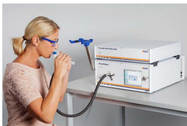
Figure 3: Handheld sampling option. Direct sampling of exhaled breath via by-pass on handheld, heated hose and sample introduction through pump.
