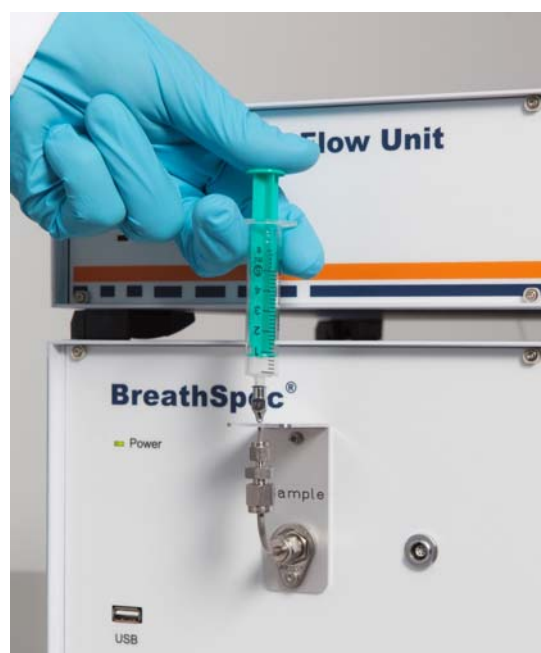
Figure 2: Sample injection into the Luer-port of the device.
