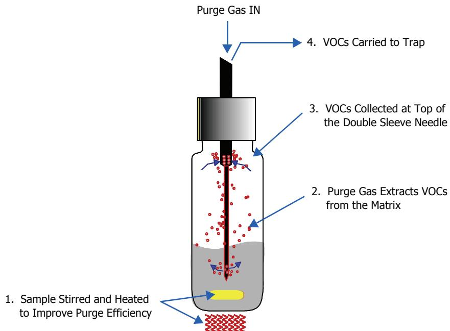
Figure 4. Vial Purging Technique
