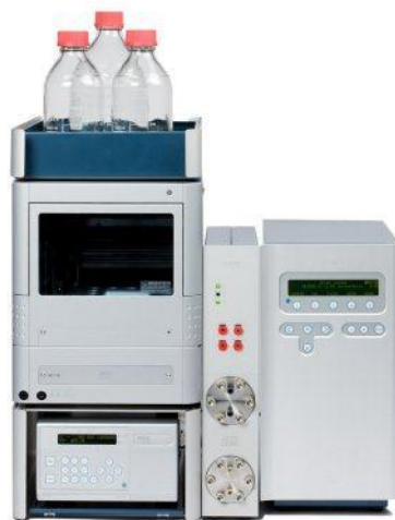
Fig. 1. ALEXYS Macrolide Antibiotics Analyzer.
