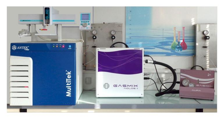
When working with LPG/LNG samples the AlyTech AURA is the ideal tool for calibration of a total Sulfur and Nitrogen analyzers. The analyzer such as the Multitek<sup>TM</sup> from PAC on the picture is connected to the GasMix<sup>TM</sup> AlOLOS in combination with AURA vaporizer. Sulfur and nitrogen can therefore be measured without the need of sample pressurization, providing a maximum operator safety.
