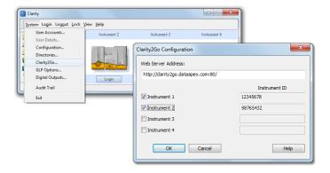
Select the instruments for monitoring, in the following example we have selected Instrument 1 and Instrument 2.
