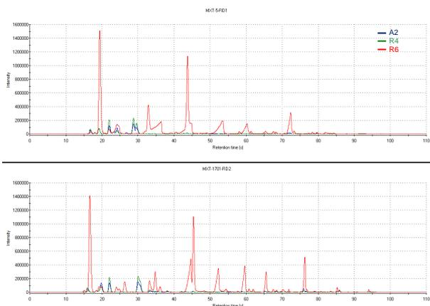
Fig.2: Volatile profile of three coconut oil samples obtained on HERACLES e-nose
