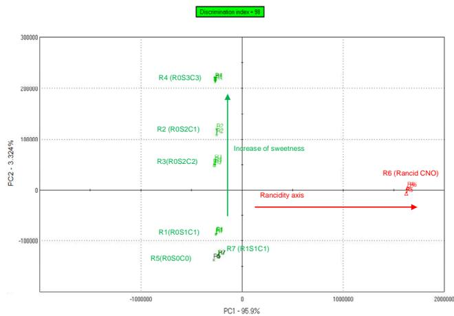
Fig. 3: Odor map of coconut oils R1 to R7 based on Principal Components Analysis (PCA) on all detected molecules
