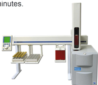
Fig. 1: Ultra Fast GC based HERACLES Electronic Nose
