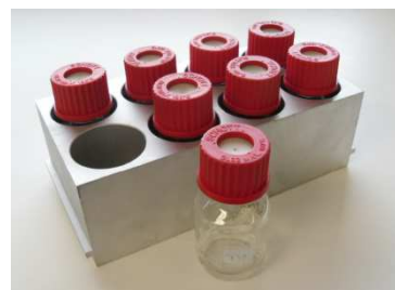
Figure 2. 50-ml vial aluminum tray for headspace generation (ref. 201-0190)
