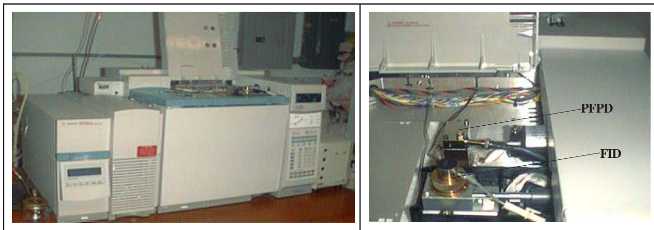
Figure 2. Photograph of the analytical instrumentation. The photograph on the right shows a close up of the Agilent FID in the front detector position (used for compound quantitation) and the OI Analytical PFPD in the back detector position (used for sulfur compound identification).
