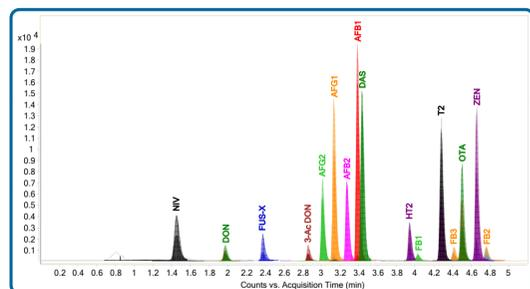
Figure 1: UHPLC-MS/MS chromatogram of a spiked corn sample (100 ng/mL) acquired with Triggered MRM with fast polarity switching.
