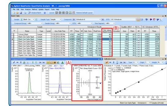
Figure 6: Screenshot of the MassHunter Quantitative software. Peak spectra are compared to library spectra (A) and library match scores are calculated (B).
