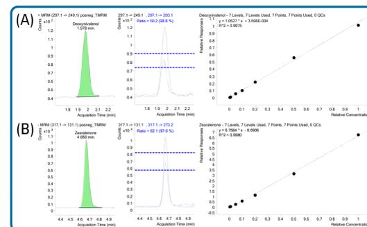
Figure 2: Chromatograms of a spiked corn extract (5 ng/mL) and calibration curves for deoxynivalenol (A) acquired in positive tMRM mode and zearalenone (B) acquired in negative tMRM mode.
