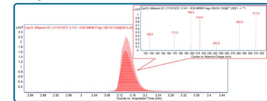
Figure 3: Primary transitions (integrated), triggered MRM transitions (5 repeats), and resulting MRM spectrum for aflatoxin G<sub>1</sub>.
