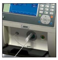
Clean the drift tube easily with the included custom brush
