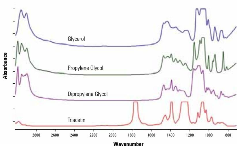
**Figure 13.** Spectra of 4 common drug additives recorded using the DialPath 30  $\mu\text{m}$  pathlength. Spectra were recorded in less than 30 seconds and results compared to reference spectra, yielding near perfect match quality.<sup>13</sup>
