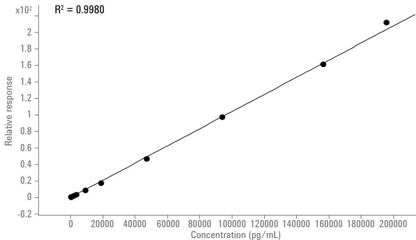
**Figure 10.** The calibration standard curve of atorvastatin measured using an Agilent 6460 LC/MS/MS System demonstrated linearity over a wide concentration range.<sup>10</sup>
