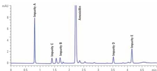
**Figure 4.** Analysis of amoxicillin and five impurities using the Agilent 1220 Infinity LC/UV System and a ZORBAX SB-Aq column.<sup>6</sup>
