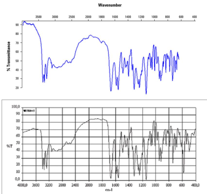
**Figure 12.** The FTIR spectra of furosemide, comparing the online spectrum from International Pharmacopoeia (Black, KBr pellet) to the one measured using the Cary 630 FTIR (Blue, DRIFT).<sup>12</sup>
