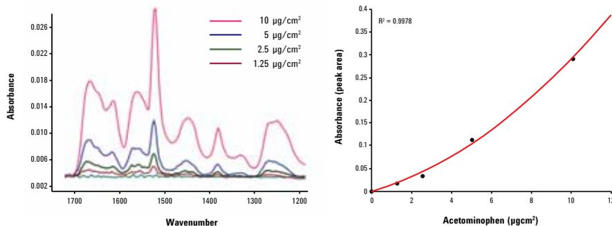
Figure 14. The cleaning validation spectra and calibration plot of acetaminophen using the 4200 Flexscan FTIR.
