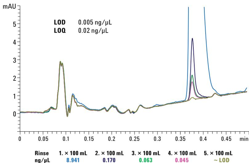
Figure 15. Residual active pharmaceutical product in equipment rinse solution after five applications of 100 mL MeOH measured with the Agilent 1290 Infinity DAD with 60 mm cell.<sup>15</sup>
