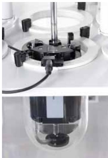
**Figure 9.** Paddle and vessel measurements taken with the Vessel Module of the 280-DS Mechanical Qualification System.<sup>9</sup>
