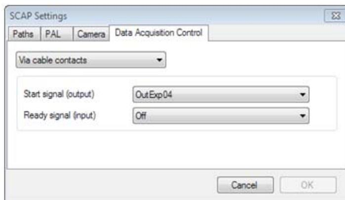
**Figure 2** Selection for start using external contact closure
