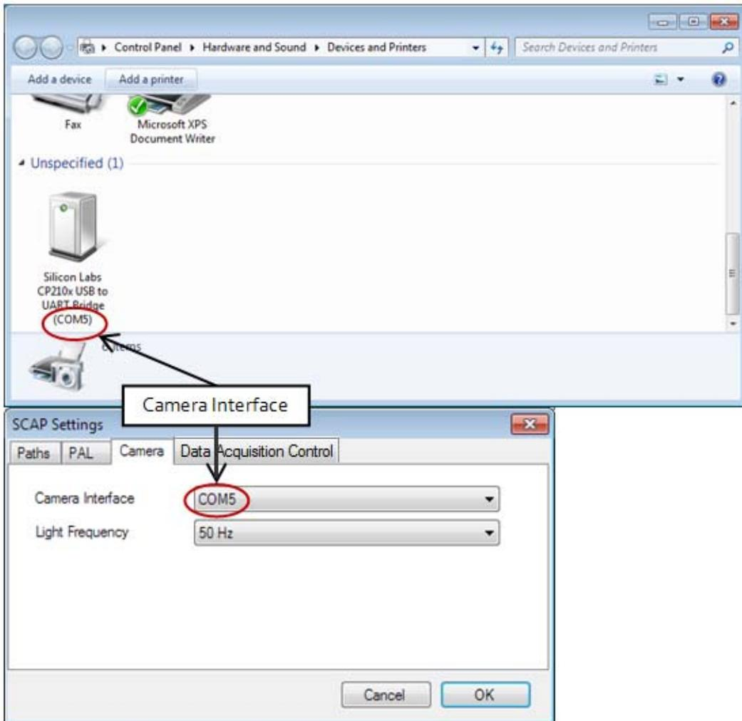
**Figure 1** Determine COM name for camera interface
