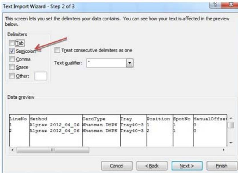
**Figure 6** Selection of format for data import in Excel
