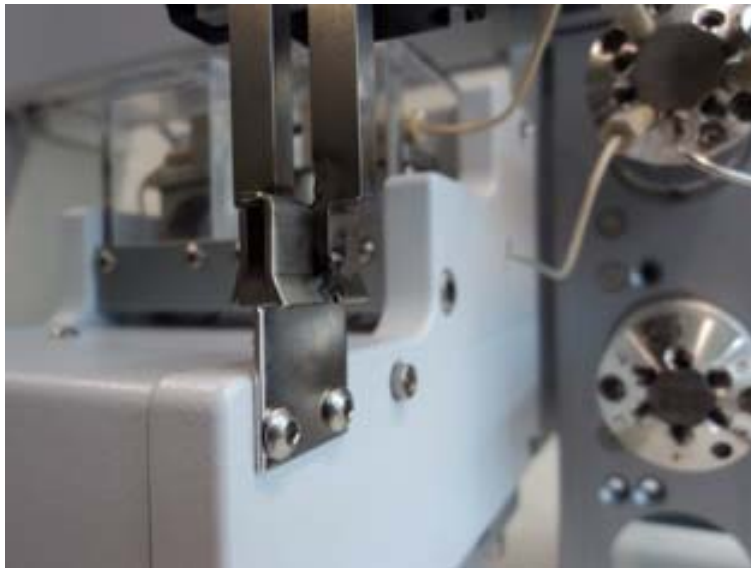
Figure 5 Position the gripper on the calibration metal plate of the clamp module
