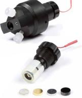
Flexcell suitable for all sorts of electrochemical analyses like the usual biogenic amines (glassy carbon), but also carbohydrates (gold), peroxides (platinum), halides (silver), sulfides (Magic Diamond) etc.
