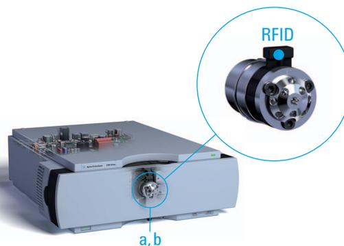
Radio-frequency identification (RFID) tags on the valve heads provide the system with details of the valve type, serial number of switches and pressure setting.
