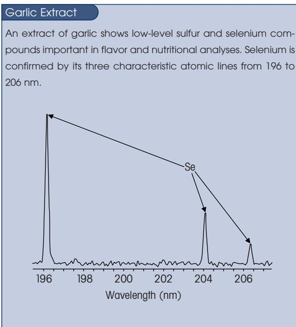
If you have any questions about the presence of an element in a chromatographic peak, an emission spectra “snapshot” helps to provide the answer.
