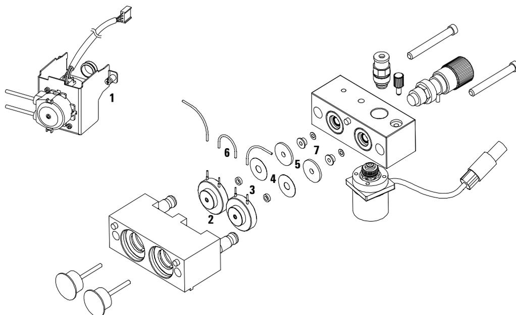
**Figure 7** Pumphead with seal wash option
