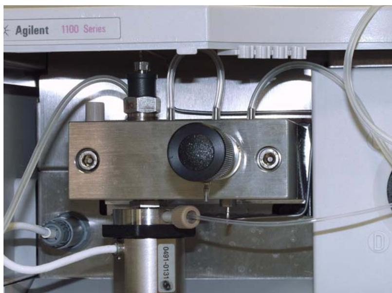
**Figure 4** Pumphead after completed installation
