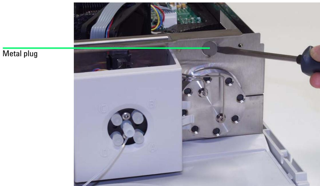
**Figure 1** Removing the metal plug from the z-panel
