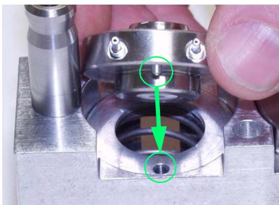
**Figure 3** Inserting the active seal wash support rings.
