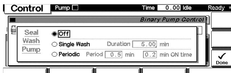
Figure 6 Example of configuration screen from the Control Module
