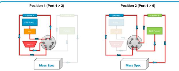
Figure 2. Back-Flush LC configuration for online sample cleanup and heart-cutting
