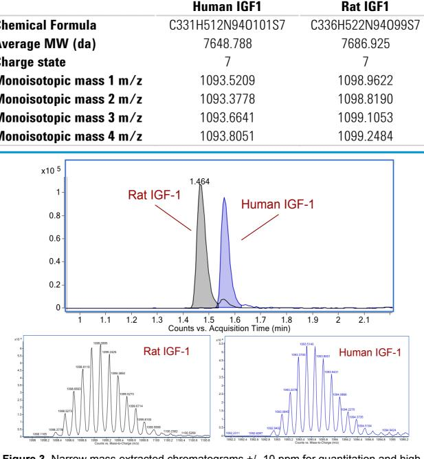
Figure 3. Narrow mass extracted chromatograms +/- 10 ppm for quantitation and high resolution mass spectra
