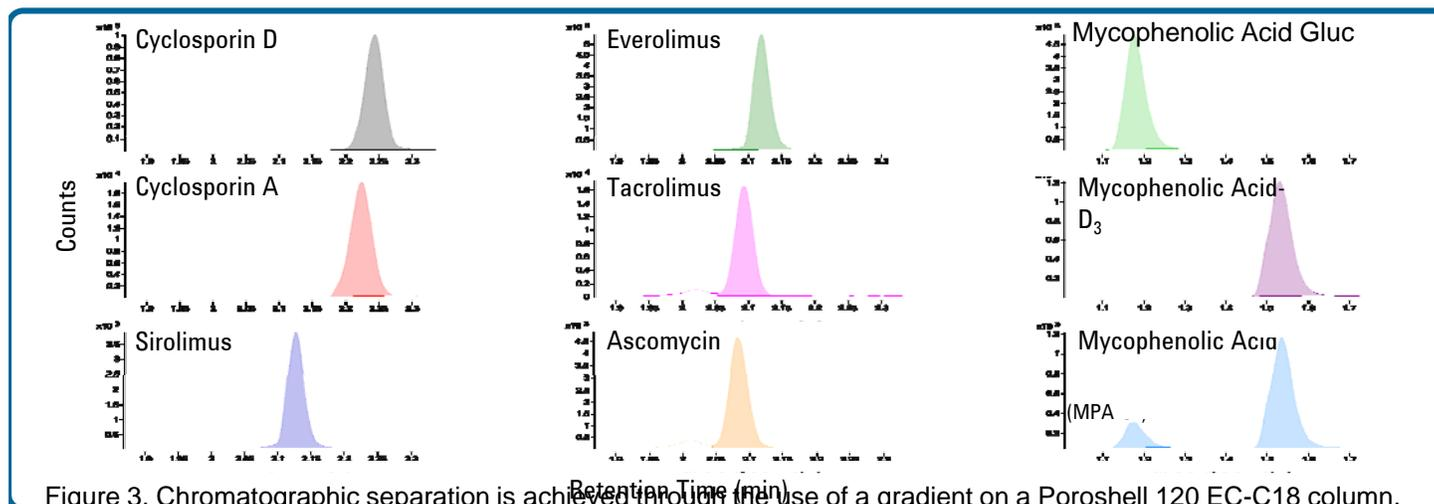
Figure 3. Chromatographic separation is achieved through the use of a gradient on a Poroshell 120 EC-C18 column.
