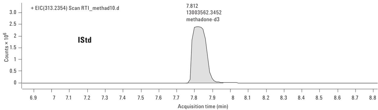
Figure 24. Methadone case sample analyzed by TOF shows detector saturation at a level greater than 1,200 ng/mL.
