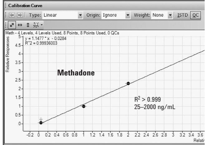
Figure 12. Linearity of compounds analyzed in postmortem samples from 25 to 1,000 ng/mL (cocaine and BE), 10 to 1,000 ng/mL (CE), and 25 to 2,000 ng/mL (methadone).
