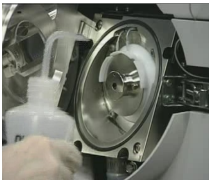
Figure 4 Rinsing the area around the spray shield
