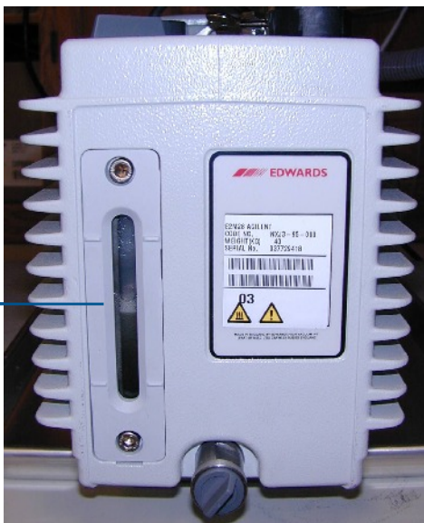
Figure 64 Fluid level window on the rough pump
