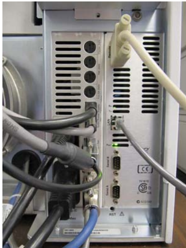
Figure 66 Disconnect the instrument power cable.
