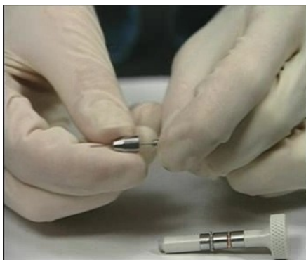
Figure 35 Installing a new needle into the collar
