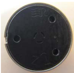
Figure 48 CDS rotor valve in its proper orientation
