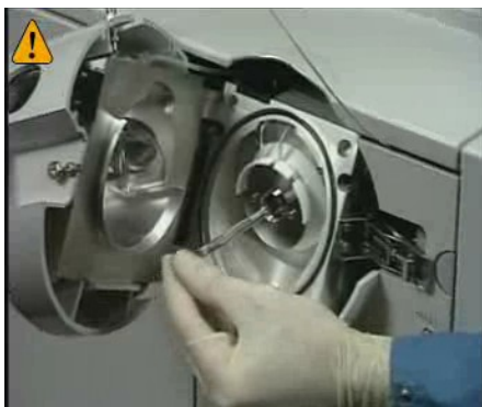
Figure 38 Reinstalling the capillary
