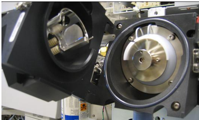
Figure 1 Opened electrospray spray chamber
