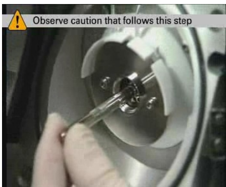
Figure 37 Pulling the capillary out of the desolvation assembly
