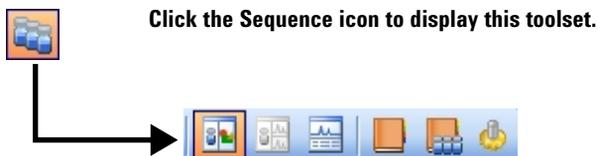
**Flow Injection Analysis (FIA)** This toolset allows you to inject multiple samples directly into the detector, which lets you bypass the chromatographic column. The results are sent to a single data file. FIA can be used for method development or for applications that do not require chromatography.
