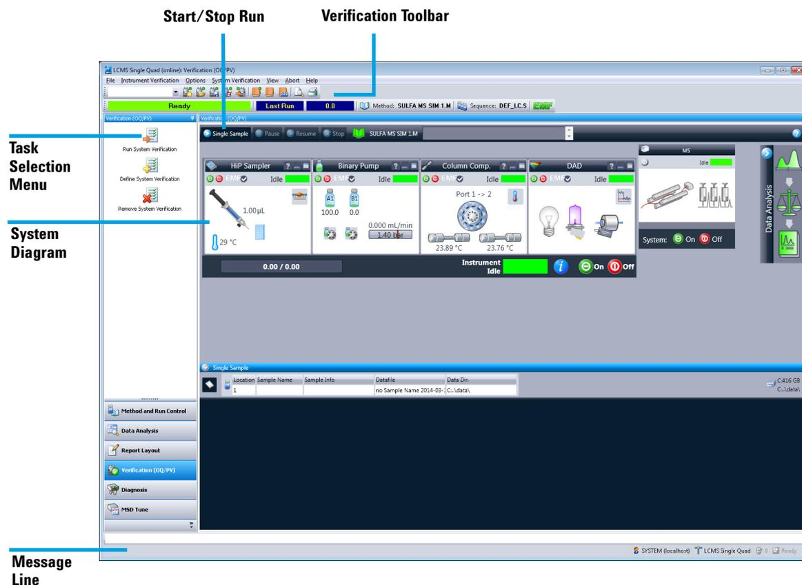
The Verification (OQ/PV) view lets Agilent service engineers test whether your analytical instruments and the ChemStation software are operating correctly according to predefined performance criteria.
