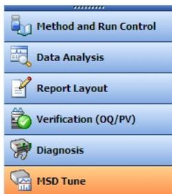
**Method and Run Control View** Allows you to set up methods and adjust instrument parameters to inject samples and acquire data one sample at a time or in automated sequences. See the next page for more information.
