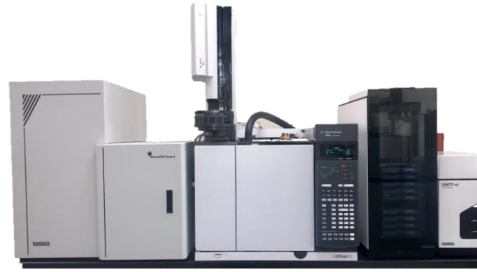
3. Sample analysis by TD-GC-TOF MS
