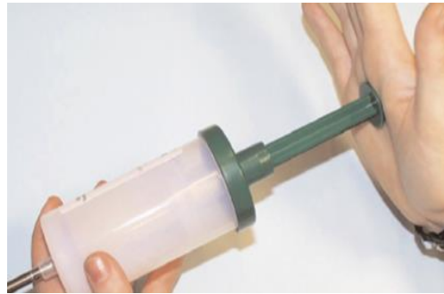
2. Transfer breath to sorbent tube
