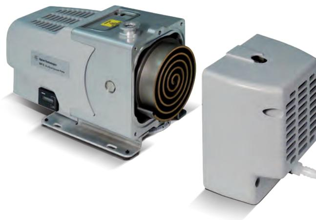
The Agilent IDP-3 dry scroll pump delivers pumping speeds of 60 l/m (3.6 m<sup>3</sup>/hr), along with very low base pressure and optimal vacuum conditions for turbo molecular pumps at equivalent gas loads.
