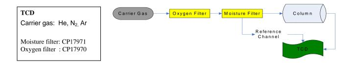
**CP-Gas Clean filters are filled with nitrogen. If you are not using nitrogen as the carrier gas, flush filters and gas lines after installation of a new filter.**
