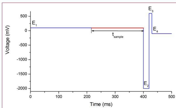
Figure 3: 4-step PAD potential waveform for the detection FDG and impurities.
