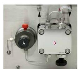
Pressure sensor (A), pump head (B) and pump head flushing (C) for automatic piston wash.
