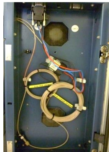
Fig. 1. PQ tubing kit installed in detector oven and connected to flow cell.
