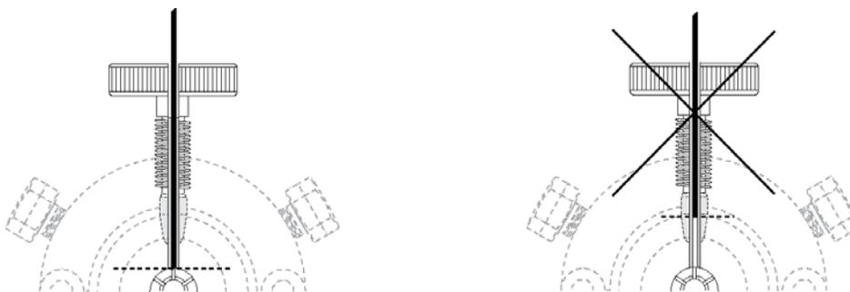
**Figure 51** Correct and incorrect Valve Needle Penetration Depth
