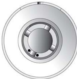
**Figure 57** Actuator Position "Active"
