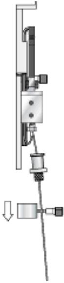
**5** Unscrew the retaining nut which tightens the holding loop to the DLW Manifold (1). Pull out the DLW Holding Loop (2).
