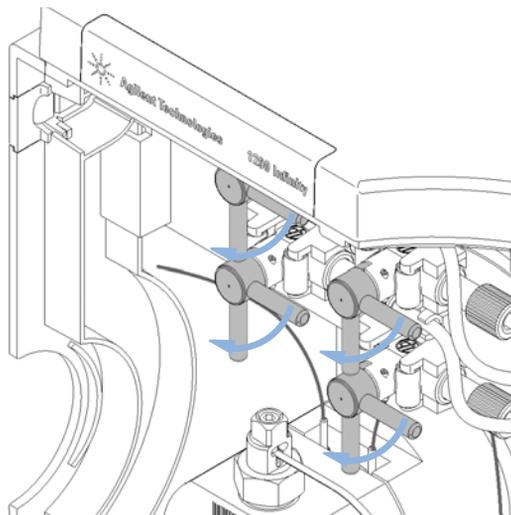
**3** Remove the flow connection between the degassing unit and the primary pump head inlet. Remove the capillary connection at the top of the secondary pump head to the pump valve. If installed, remove the tubings of the seal wash option.
