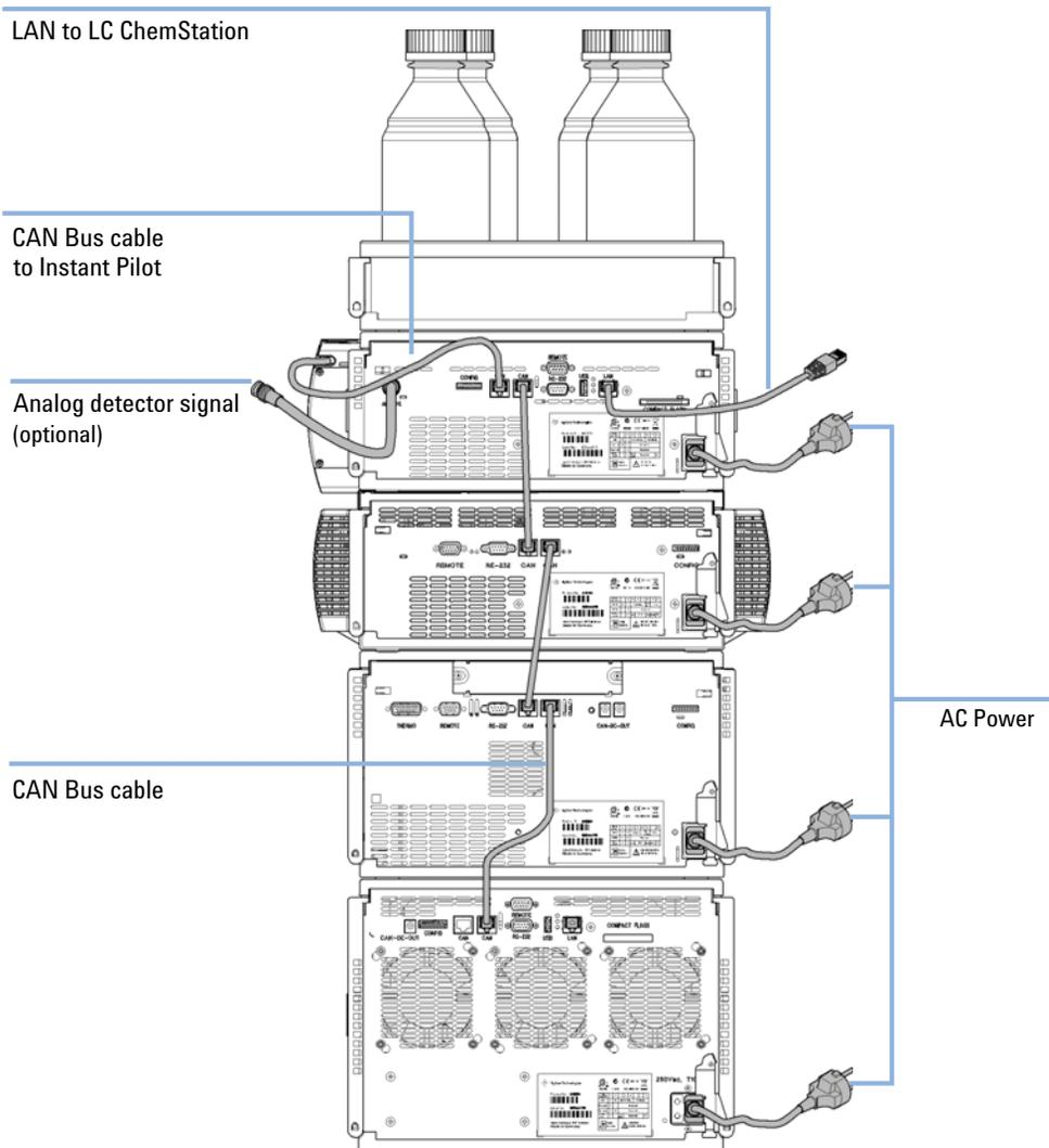
**Figure 4** Recommended stack configuration 1290 Infinity (rear view)
