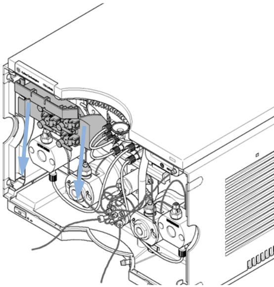
**4** After replacing the panel or after completion of other maintenance, re-install the panel and all flow connections.
