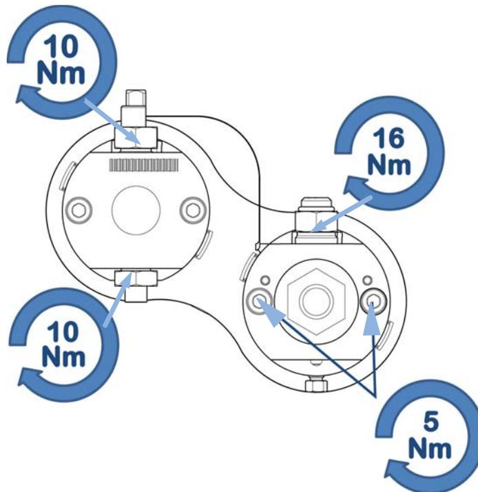
**Figure 20** Overview of torques for pump head procedures
