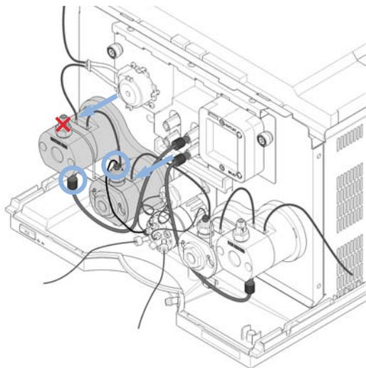
DO NOT REMOVE the capillary connection between the pump heads marked by the red X.
