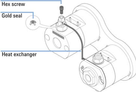
**4** Unscrew the outlet valve with a 14 mm wrench.
