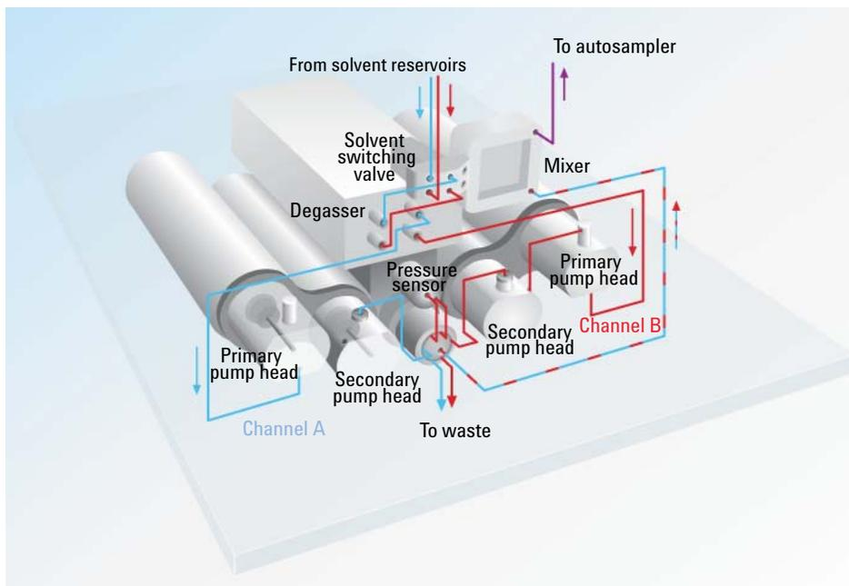
**Figure 19** Flow Connections
