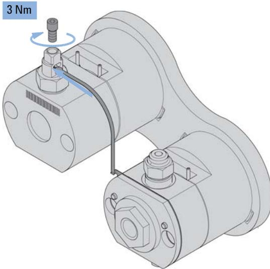
**20** Install flow connections.
