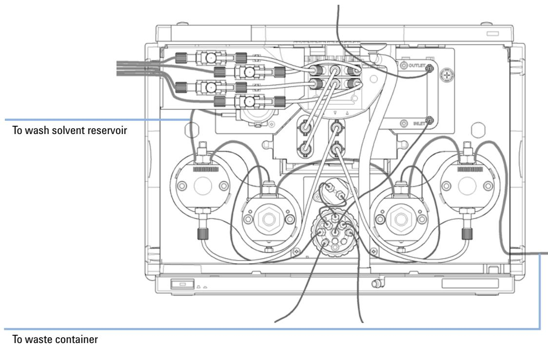
**Figure 12** Binary Pump with Seal Wash Function
