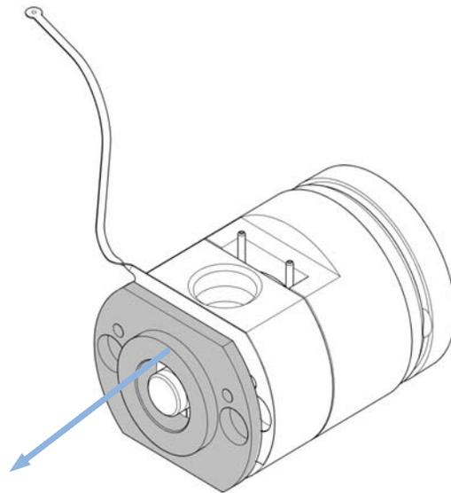
**3** Remove the screw at the bottom of the pump head. Do not drop the golden spacer fitting.
