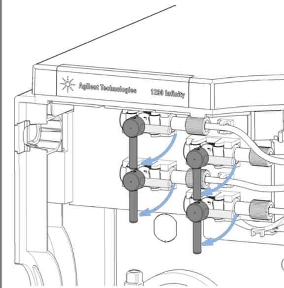
**2** Lift up the capillary and remove it from the primary pump head.
