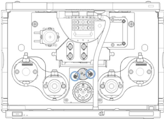
**6** Connect the capillaries from the valve to the pressure sensor: connect port 3 to the pressure sensor inlet and port 2 to the outlet.
