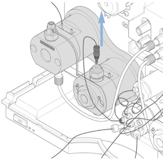
**2** Unscrew the tubing at the inlet valve.
