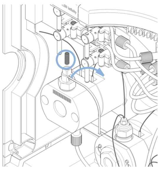
**3** A gold seal between outlet valve and heat exchanger capillary is used for a tight connection. The seal can be replaced separately as needed.
