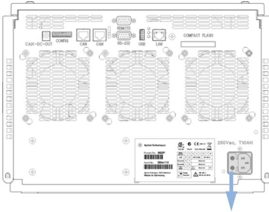
**2** Install the new fuse 10A to the carrier and insert the carrier to the fuse compartment.
