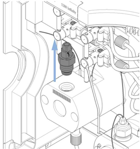
**5** Insert the outlet valve into the pump head. Using a torque wrench, set 10 Nm and close the outlet valve.
