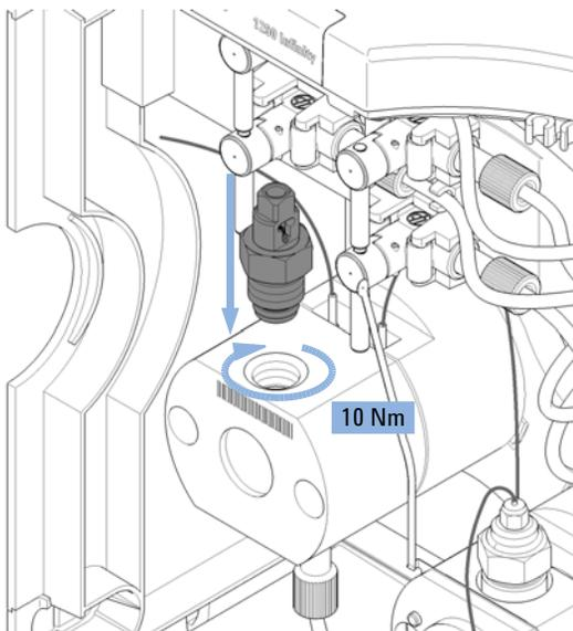
**6** Insert the heat exchanger capillary into the outlet of the outlet valve. Using a torque wrench with a 2.5 mm hex bit, set 3 Nm and close the hex screw at the top of the outlet.
