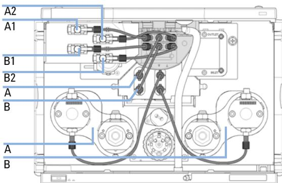
**2** Push down the SSV panel for removing it.
