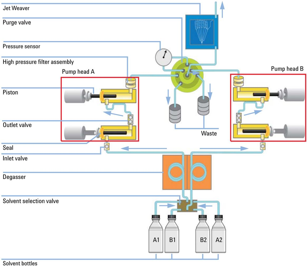
**Figure 1** The hydraulic path
