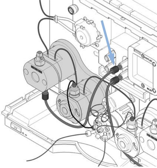
**8** Reinstall the capillary connection to the High Pressure Filter Assembly.
