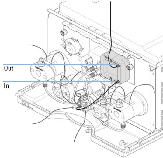
The inlet at the bottom of the Jet Weaver is connected to the central port of the pump valve by a capillary (length 300 mm, 0.17 mm i.d.). The outlet at the top is connected to the autosampler.
