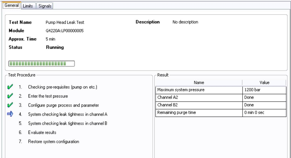
**Figure 16** Pump Head Leak Test – Results
