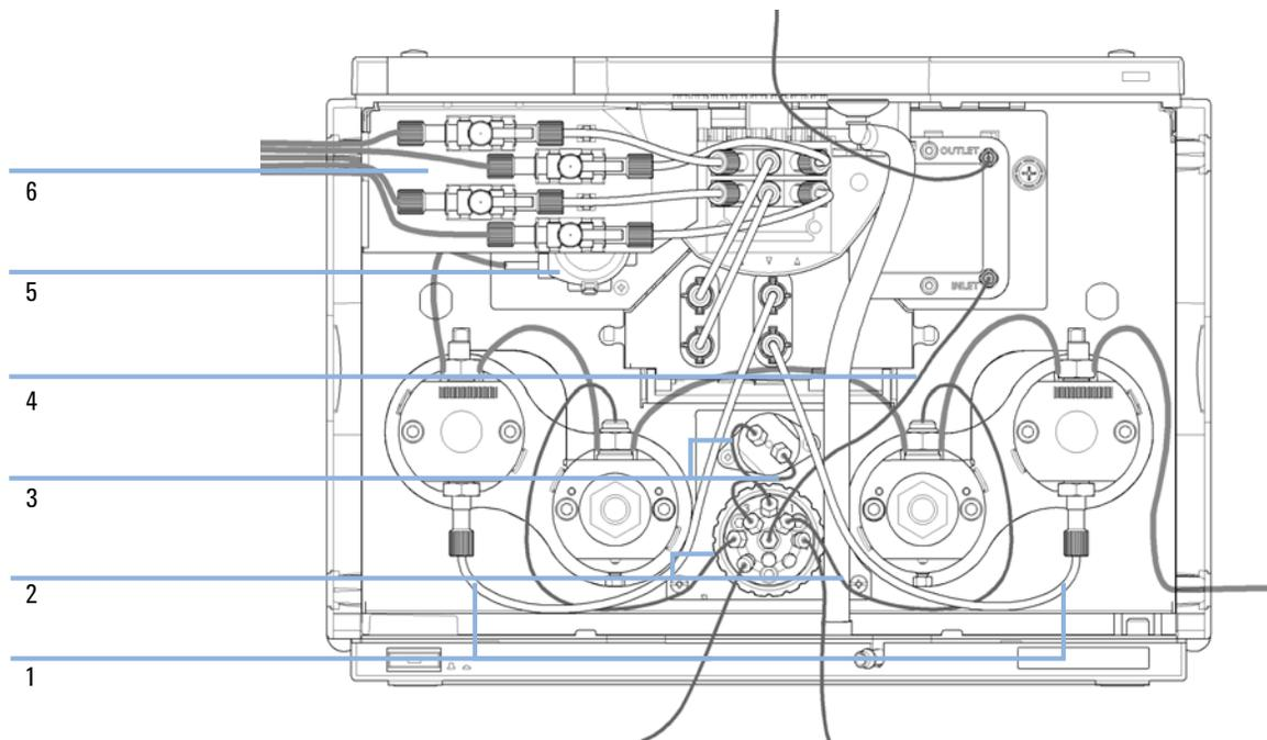
**Figure 23** Flow connections of the pump
