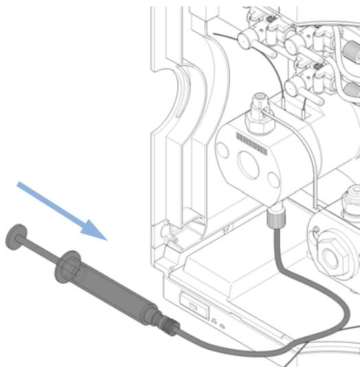
**7** Detach the syringe and reconnect the tubing into the degassing unit.
