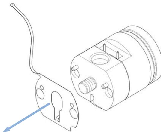
**5** If removed, first insert the spacer fitting. Then insert the new heat exchanger to the opening in the pump head and lift it over the pins.
