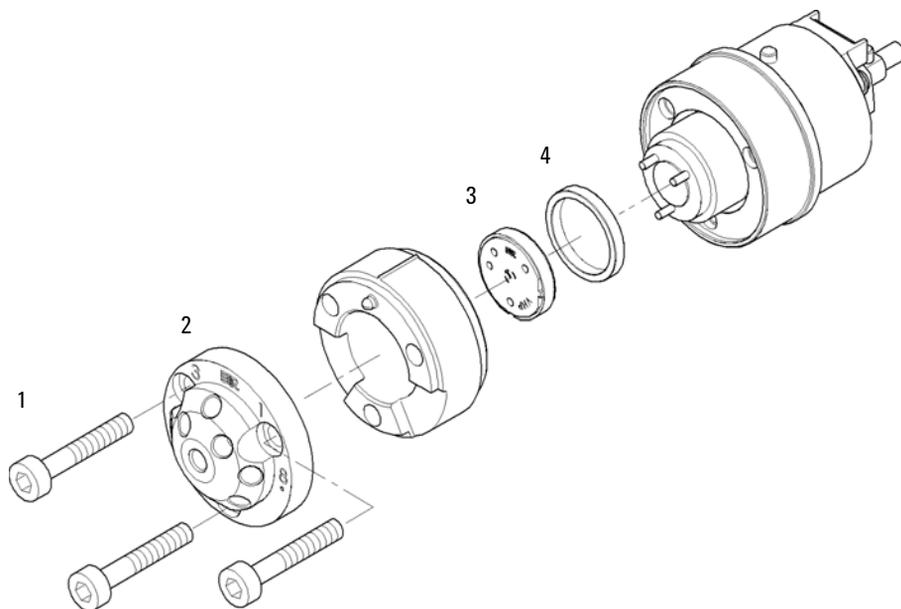
**Figure 31** Purge valve parts
