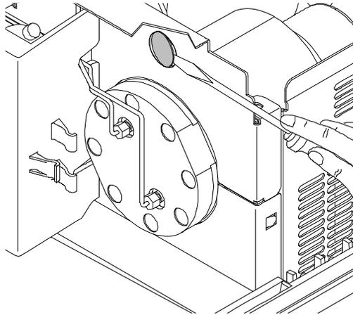
**Figure 20** Removing the metal plug from the z-panel
