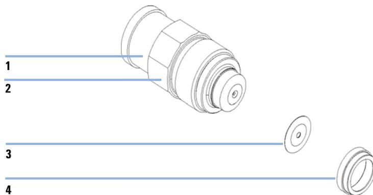
**Figure 29** Outlet Ball Valve Assembly
