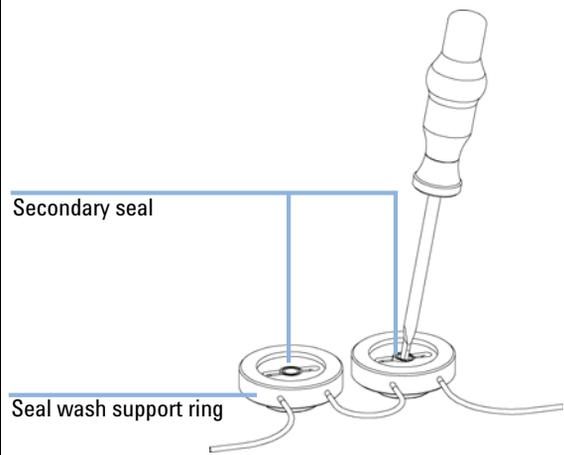
**5** Using the insert tool press the secondary seal (spring pointing upwards) into the recess of the support ring. Place a seal wash gasket in the recess of the support ring.
