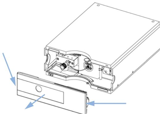
**Figure 9** Removing the Front Cover
