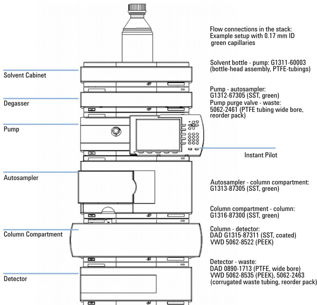
**Figure 5** Recommended Stack Configuration (Front View).
