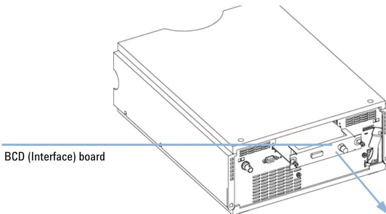
**Figure 24** Exchanging the Interface Board
