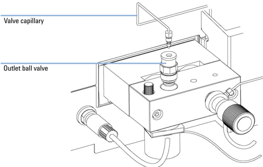
**Figure 17** Exchanging the Outlet Ball Valve
