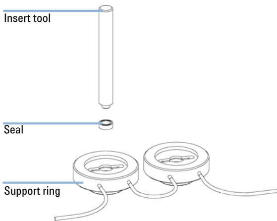
**6** Place the support rings on the plunger housing (plungers not installed) and snap the pump head and plunger housing together.
