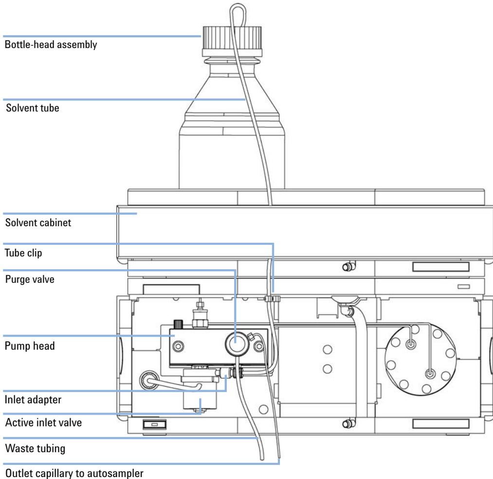
**Figure 10** Flow Connections of the Isocratic Pump
