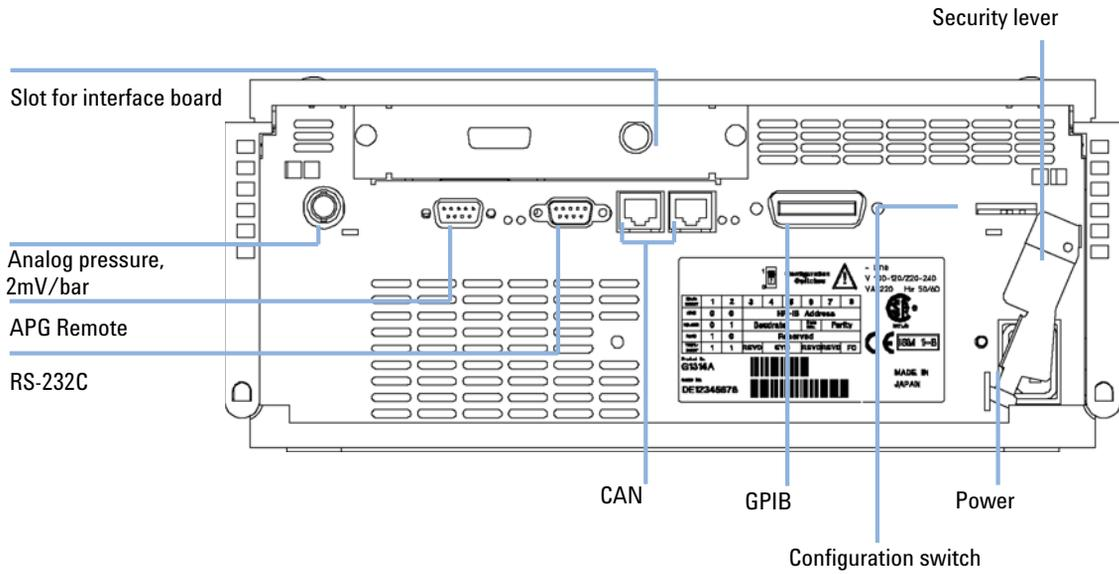
**Figure 4** Rear View of Pump - Electrical Connections and Label
