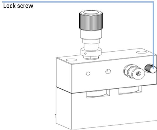
**9** Slide the pump head assembly onto the metering drive. Apply a small amount of pump head grease to the pumphead screws and the balls of the spindle drive. Tighten the pumphead screws stepwise with increasing torque.
