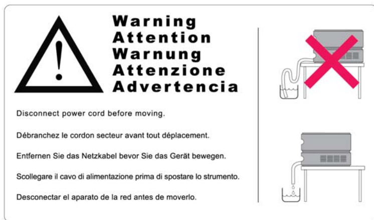
Figure 13 Warning label (illustration for correct waste tubing)
