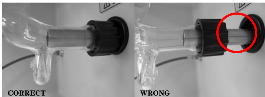
Figure 12 Fixing the Tip of Nebulization chamber
