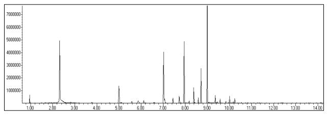
Figure 3: Total Ion Chromatogram (TIC) of VOCs present in a Banana (baby food) sample.
