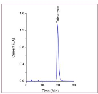
Figure 4:  $20~\mu L$  injection of  $100~\mu g/mL$  Tobramycin sample solution in mobile phase (sample solution (b) as described in EP monograph) for the Tobramycin assay analysis.
