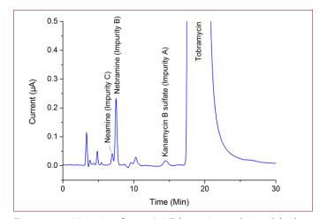
**Figure 1:** . 20 μL injection of a 1 mg/mL Tobramycin sample in mobile phase (Test solution (a) as described in the EP monograph).
