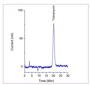
Figure 3: 20  $\mu$ L injection of 2.5  $\mu$ g/mL Tobramycin CRS in mobile phase (reference solution (b) as described in EP monograph).
