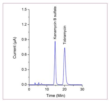
**Figure 2:** 20  $\mu$ L injection of a standard consisting of 0.05 mg/mL kanamycin B and 0.05 mg/mL Tobramycin CRS in mobile phase (Reference solution (d) as described in EP monograph).
