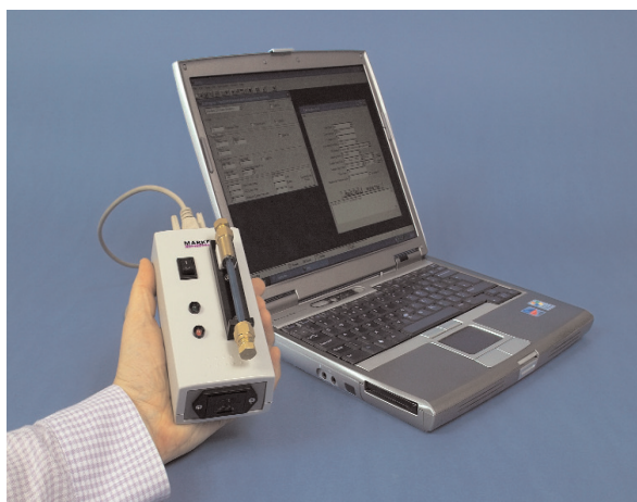
Figure 4: The TAG SCRIBE field-portable device, used with PC for programming tags in the field or laboratory
