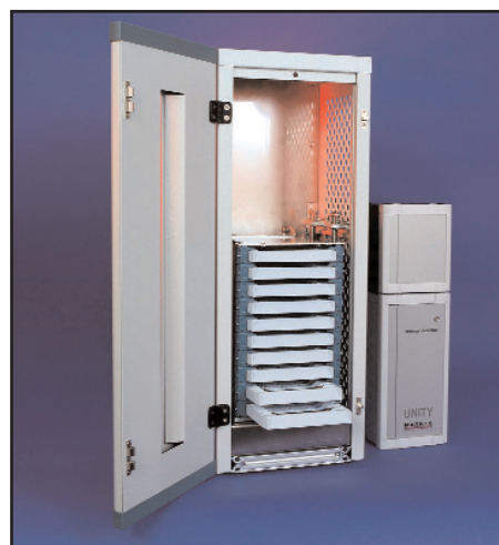
Figure 4: ULTRA-UNITY automated thermal desorber for up to 100 tubes
