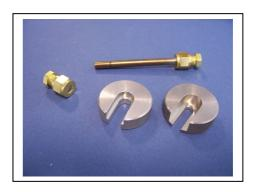
2. The two halves of the CapLok tool are slightly different. The disk etched with the Markes Logo should be used on the top of the cap and the other disk should be used over the tube on the nut end
