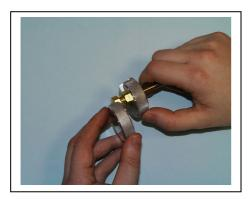
3. Loosen the brass cap using the CapLok tool as shown (by twisting the two discs in opposing directions). Then pull the nuts from the end of the tubes.
