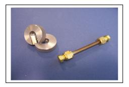
1. CapLok tool and sorbent tube capped with ¼ inch brass SwageLok type long-term
