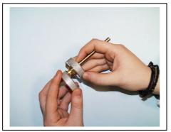
5. To replace the caps, push them onto the end of the tube and tigten until finger tight. Use the CapLok tool (by twisting the two discs in opposite directions) to tighten the nut a further quarter to half turn.
