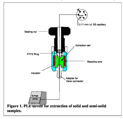
respectively. Isolation achieved by a ceramic ring around the stainless-steel ring [12]. The temperature was programmed by defining a temperature, start a temperature rate, a temperature and a hold time controller. The temperature programme was manually started at the beginning experiment. A Phoenix 20 CU syringe
