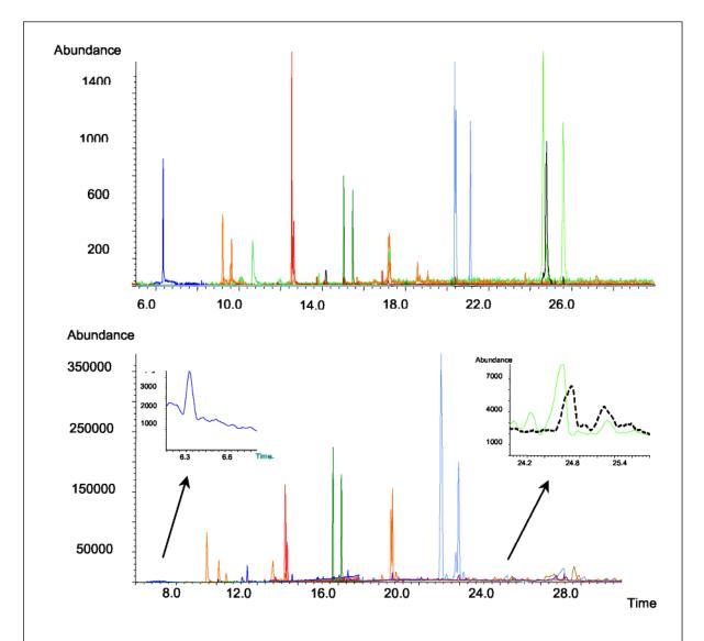
Figure 4. LVI–GC–MS of (A) standard solution of PAHs (concentration, 5 ng/ml) and (B) PLE extract of the non-spiked organic soil. For selected m/z values and other experimental details, see Table 1 and text.
