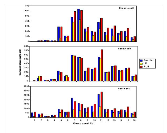
Figure 3. PAH concentrations determined by LVI-GC-MS in three samples after Soxhlet or liquid-partitioning. The concentrations were calculated from three separate analyses of each sample. See Table 1 for peak identification.
