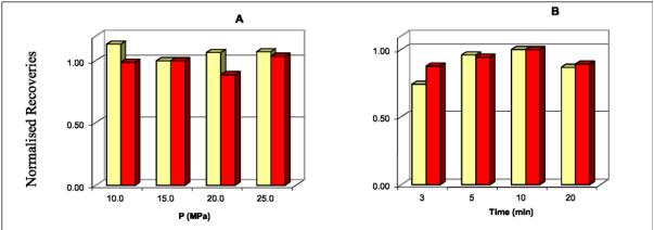
Figure 2. Influence of (A) extraction pressure and (B) extraction time on the recoveries of naphthalene ( ) and pyrene ( ) spiked to an organic soil at the 75 ng/g level. The recoveries were normalised against the yields found when the soil was extracted with toluene for 10 min (A) at 180°C and 15 MPa, and (B) at 200°C and 15 MPa.
