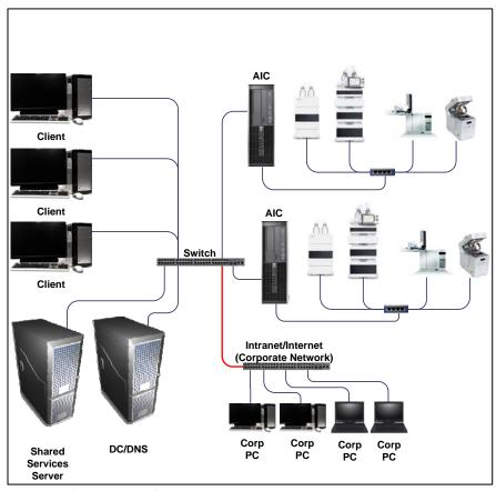
Figure 1 Sample client/server topology: Network Isolation
