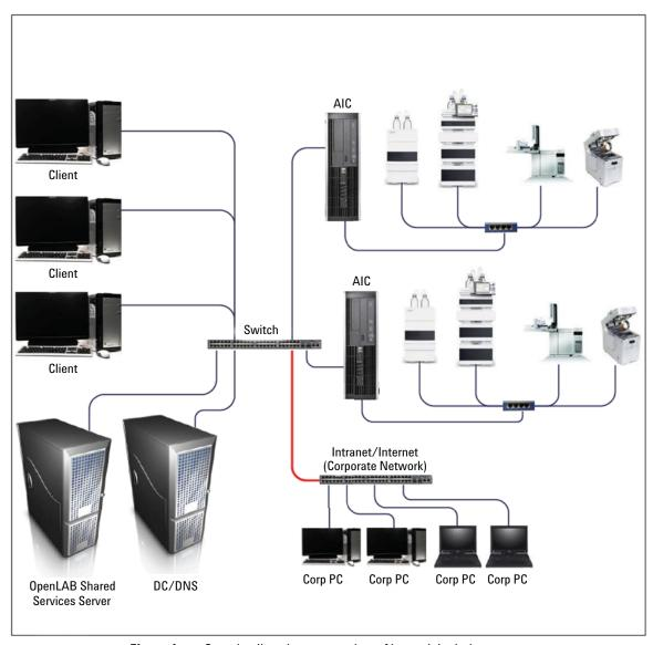
Figure 1 Sample client/server topology: Network Isolation
