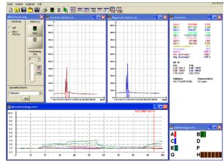
Bild 5: Analisis from WinMuster and the response from the GDA to the detection of methyl bromide.
